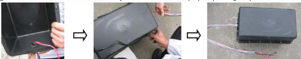
Pass wires through the connector
